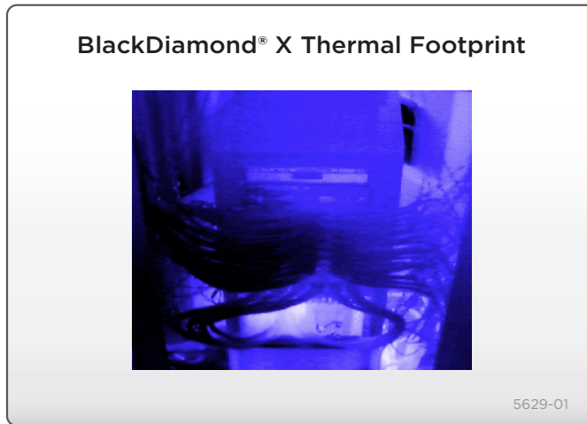
Figure 4: BlackDiamond X Series Thermal Footprint – chassis running cool (blue) in upper part of picture, with 'hot' chassis, a test platform, (white) in lower part.
